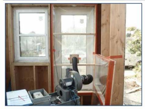
Comments/Observations: Master Test 1 is the initial assessment of Specimen 1, a Euroline-brand door measuring 40" x 86 ½ ". Prior to testing, a purge was run to remove debris and/or moisture from the test area. Master Test 1 tested Specimen 1 at 6.00 psf. Technicians did not observe any water intrusion during the test and Specimen 1 received a Pass.
