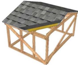
b) 4:12 Slope roof with roofing felt underlay
