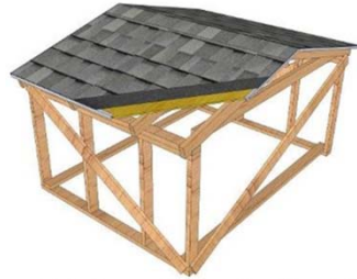
a) 3:12 Slope roof with roofing felt underlay
