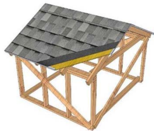
c) 6:12 Slope roof with roofing felt underlay
