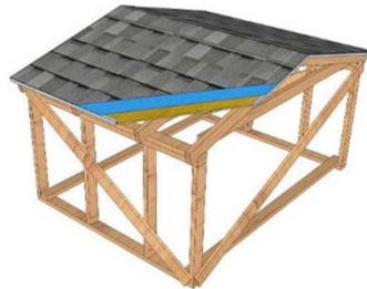
d) 3:12 Control roof with SAM underlay
